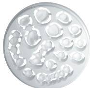
Semi-finished components of various materials for the dental sector can be made by means of milling processes and CAD-CAM technologies. The work flow entails scanning and digitalizing of the model, the check of the passive fit of the structure by probing and finally producing it in a highly precise and repeatable way with 5 axis machines.
